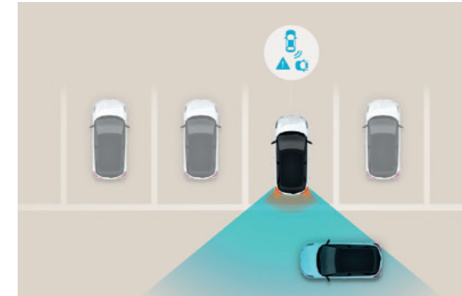
Rear Cross-Traffic Collision-Avoidance Assist (RCCA). Perfect for parking lots. When reversing out of areas with low visibility, the system not only warns the driver if vehicles approach from the side – it also applies the brakes automatically.
